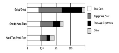
Figure 1: Cost Comparison of Turning versus Grinding [3]
